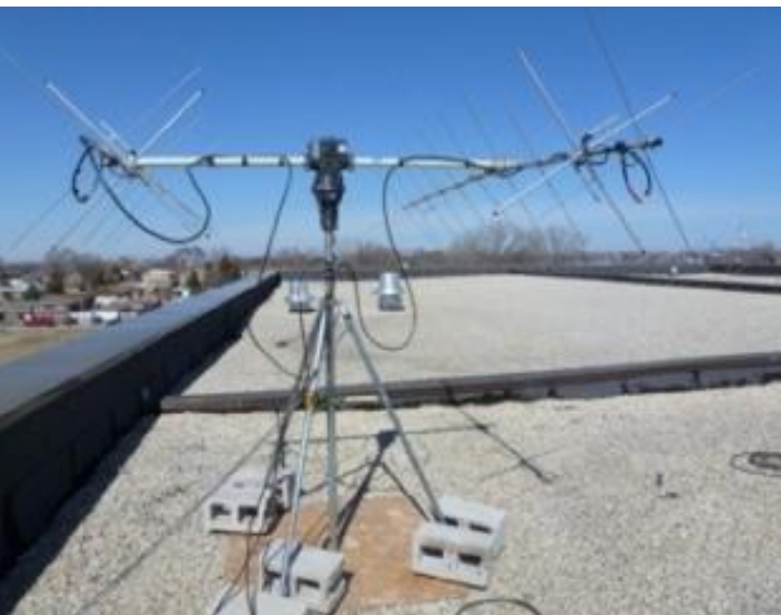
One of the several antennas on the roof of the school. It has azimuth and elevation motion to track the space station.
