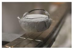
resistance of the copper, and so rather than stopping, the magnet slowly moves down the pipe. However, when one uses a superconductive material, the magnet doesn't move. It just floats, suspended. Why? The superconductor has no resistance, so the current, and thus the magnetic field, do not dissipate, and the magnet essentially levitates on the field it induced (See photo).
