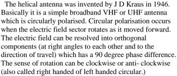
In most cases helical antennas will need to work against a ground plane, though this is not always the case. The ground plane can be flat or cupped in the form of a cylindrical cavity or in the form of a frustrum cavity. The antenna is fed by coaxial cable, the central conductor being connected to the helix at the feed point and the outer conductor attached to the ground plane. Westlakes Amateur Inc.- Magazine September 2013
