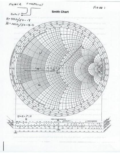
distance at the center of the top line, Point "G," and looking to the left, to "0" on your ruler, you will determine the SWR, by reading the corresponding number at that point, Point "H," which in this case, is an SWR of 7:1.
