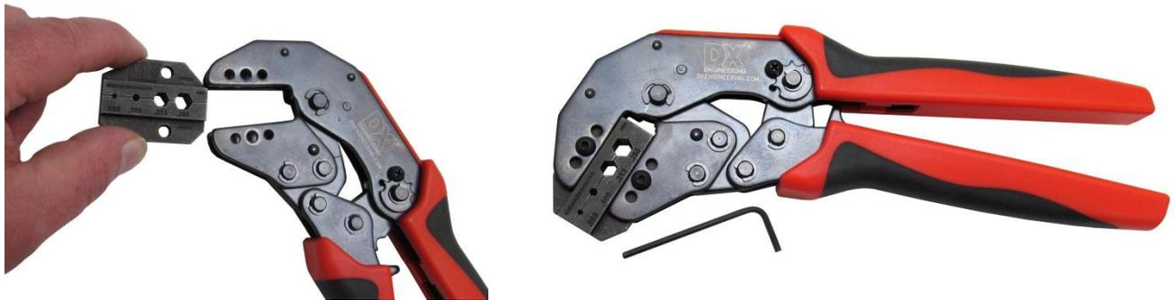
When installing the Powerpole® Die Set, use the supplied longer screw and Nyloc Nut and washer to allow for the addition of the Powerpole® crimp connector holder.
