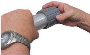
DX Engineering recommends the **DXE-UT-KIT-DBR Tube Deburring Tools**, **DXE-22166 Slim Grip Deburring Tool**, or the **DXE-22600 Deburring Tool with Extending Handle and Extra Blades** for this operation.
