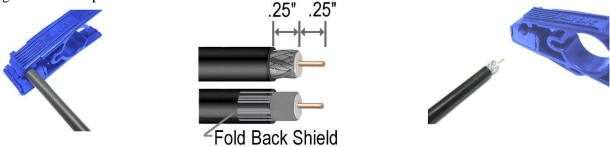
Fold the braided shield back onto the outer jacket.
