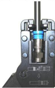
4. Fully squeeze the **DXE-SNS-CT1** Compression Tool handles together to completely compress the **Snap-N-Seal®** connector as shown.
