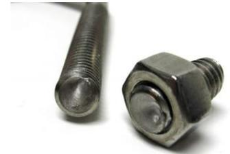
Sometimes this is referred to as “cold welding”. Anyone who has had or seen a bolt and nut with this problem can understand this description. It’s not cheap hardware; it’s the lack of common preventative measures that should be taken when using stainless steel hardware.
