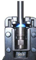
5. Remove completed coaxial cable assembly from **DXE-SNS-CT1** Compression Tool.
