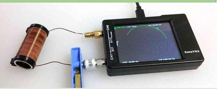
Testing a coil's impedance, resistance, or reactance.
